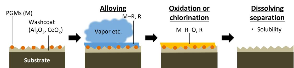
Technology to dissolve precious metals in non-oxidizing acids (e.g., hydrochloric acid) and solutions (e.g., sea water) using a pretreatment of alloying them with reactive metals such as magnesium (Mg) or calcium (Ca) followed by oxidation or chlorination.
