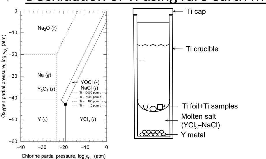
Based on thermodynamic calculations, we have developed a novel deoxidation technology of directly removing oxygen from Ti scrap using rare earth metals such as yttrium (Y) and cerium (Ce).
