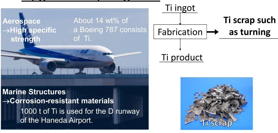
Titanium (Ti) scrap generated in the Ti ingot fabrication process is contaminated by oxygen impurities. Therefore, it is difficult to recycle Ti scraps into ingots.
