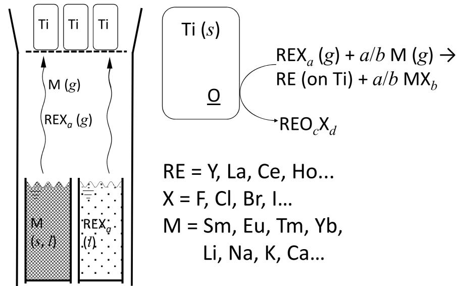
We have developed a novel deoxidation technology for reducing the amount of deposits on Ti surface and impurities in Ti by supplying deoxidants and fluxes to Ti through the gas phase.
