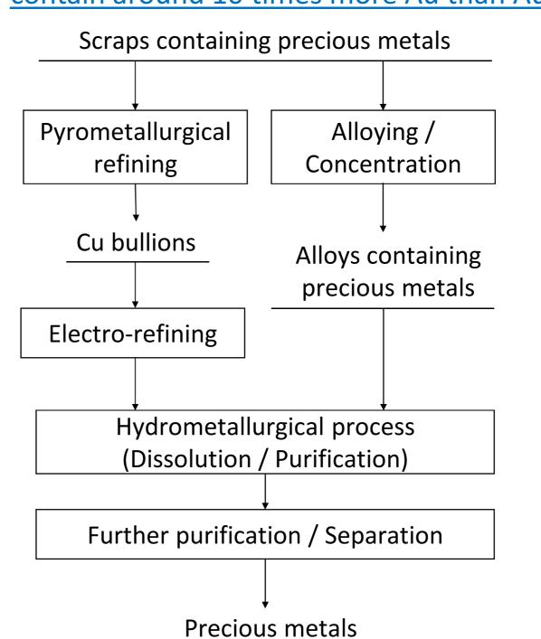
To dissolve precious metals into solution, the process
