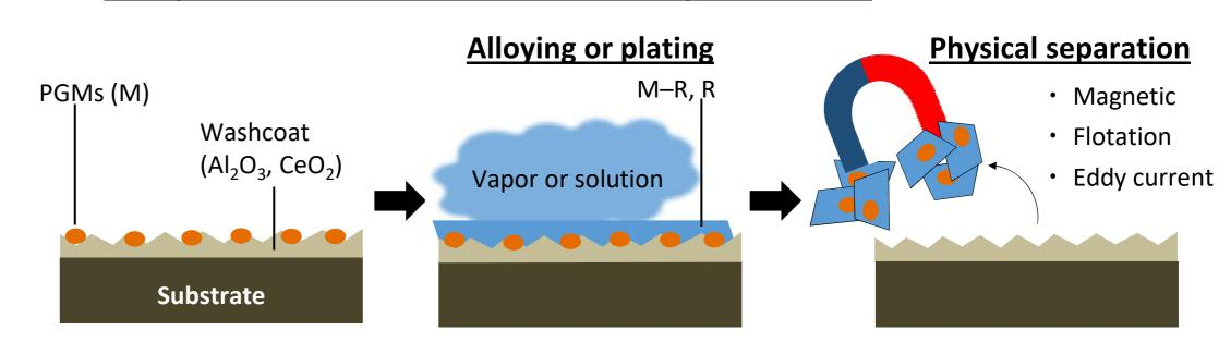
Technology to selectively add functions (e.g., magnetism, hydrophobicity) to areas of scrap containing precious metals by electroless plating or chemical treatment with chloride or sulfide vapors, allowing for the concentration of precious metals using physical separation.
