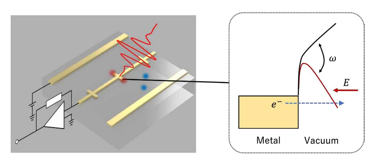
The intense optical field of infrared ultrashort pulses can control electron wave packets on the attosecond scale. We are developing a detector that can catch up with optical frequencies beyond 100 THz in combination with the field enhancement properties exhibited by metallic nanostructures.
