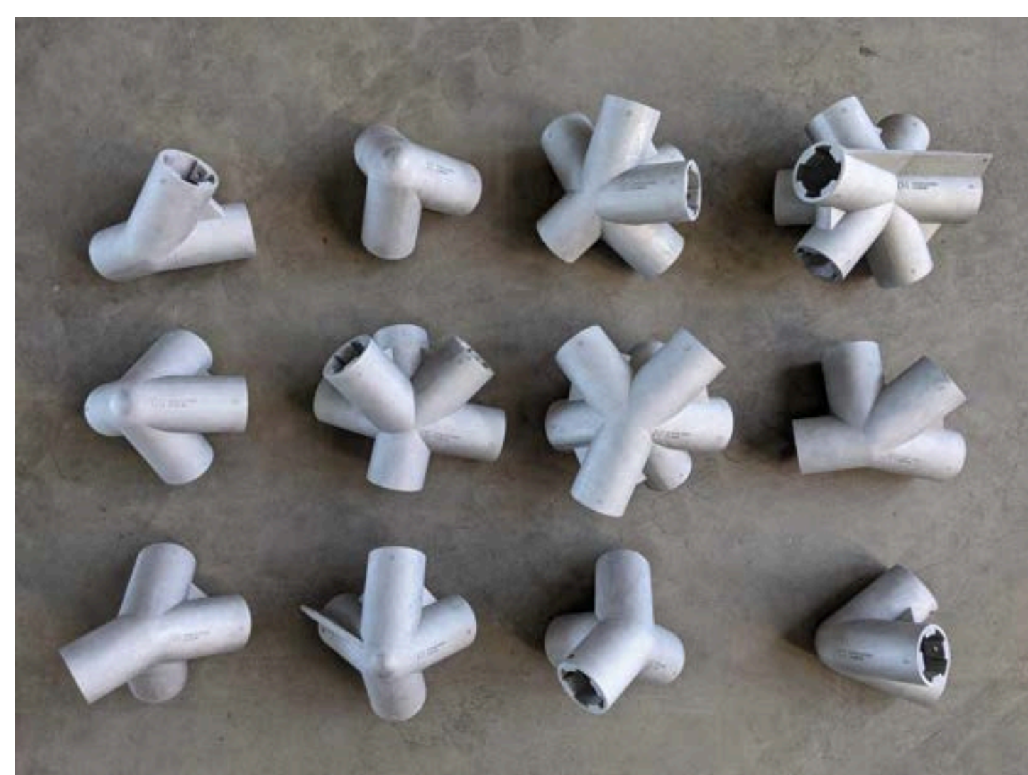
AM Joints with customized outputs depending on the specific angles at which the pipes are attached
