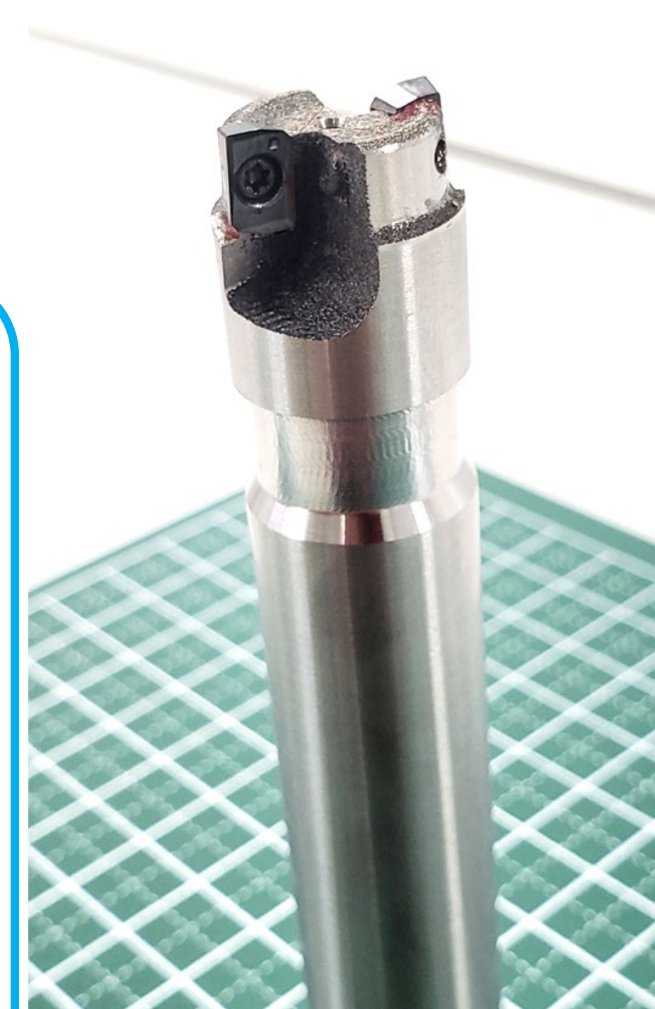
Appearance of the manufactured tool Ejection from the coolant hole built into the tool
