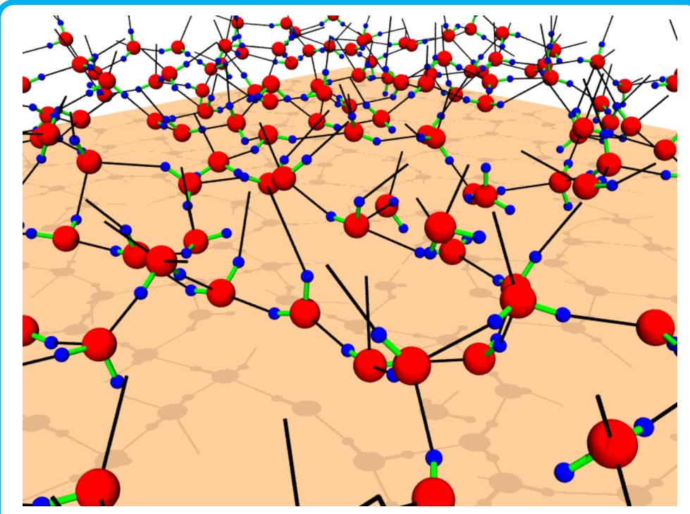
Simulations of H<sub>2</sub>O/ice phase transitions in water films near solid surfaces
