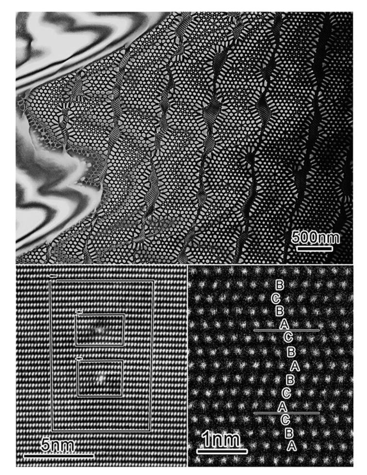
Fig. 3. Screw dislocation network ( $\alpha$ -Al<sub>2</sub>O<sub>3</sub>), dislocation core structure ( $\alpha$ -Al<sub>2</sub>O<sub>3</sub>), stacking fault
