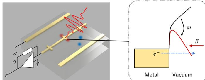
The intense optical field of infrared ultrashort pulses can control electron wave packets on the attosecond scale. We are developing a detector that can catch up with optical frequencies beyond 100 THz in combination with the field enhancement properties exhibited by metallic nanostructures.
