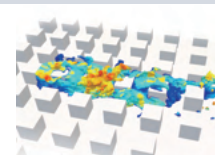
Computational prediction of pollutant dispersion in block-arranged urban model
