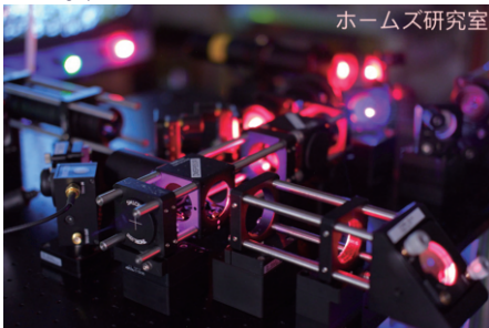
Optical setup used for single-QD measurements
