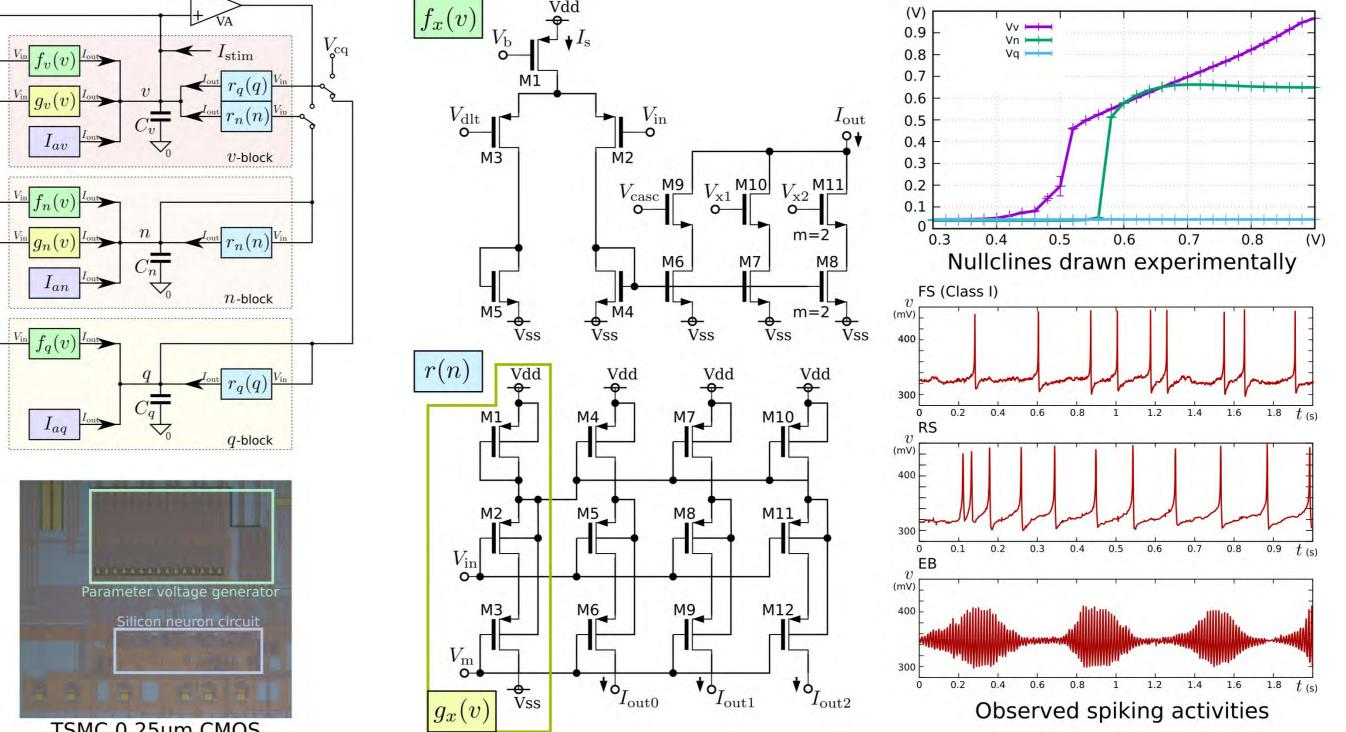
7nW / neuron 2pW / synapse **0.25µm CMOS process Power supply voltage 1V**
