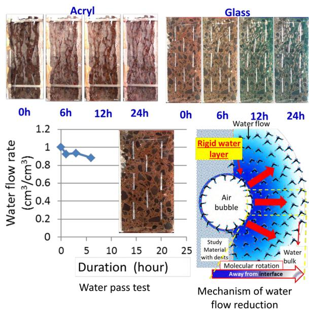
Water flow reduction due to generation of air bubble
