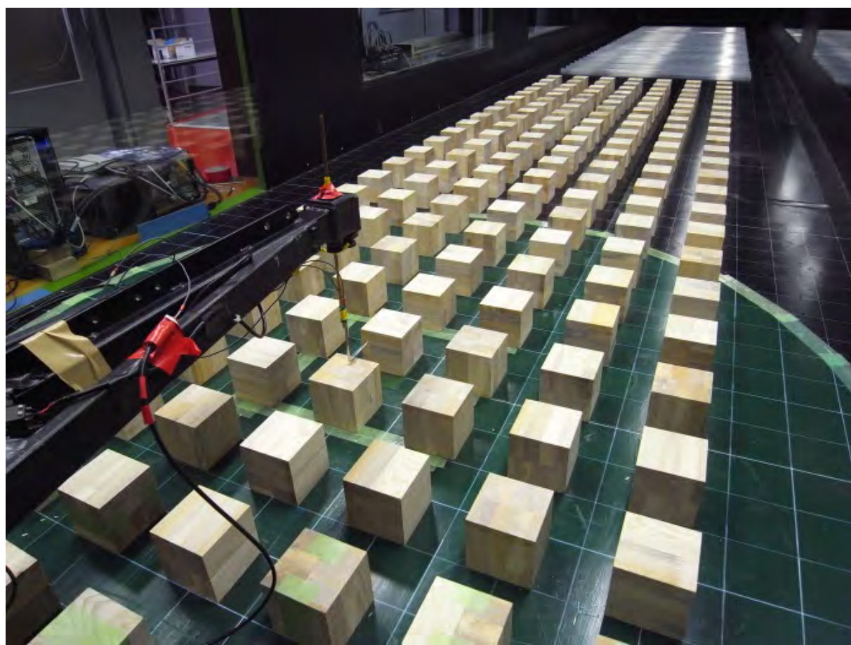
Wind tunnel experiment of city airflow
