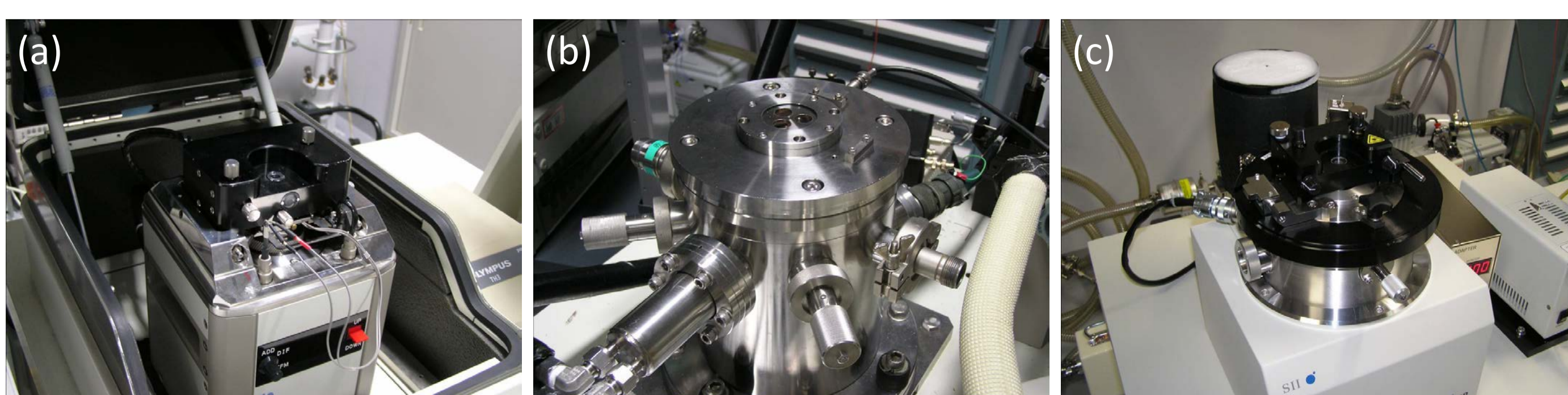
Multi-functional SPM equipments: (a) air type, (b)/(c) high vacuum and variable temperature type
