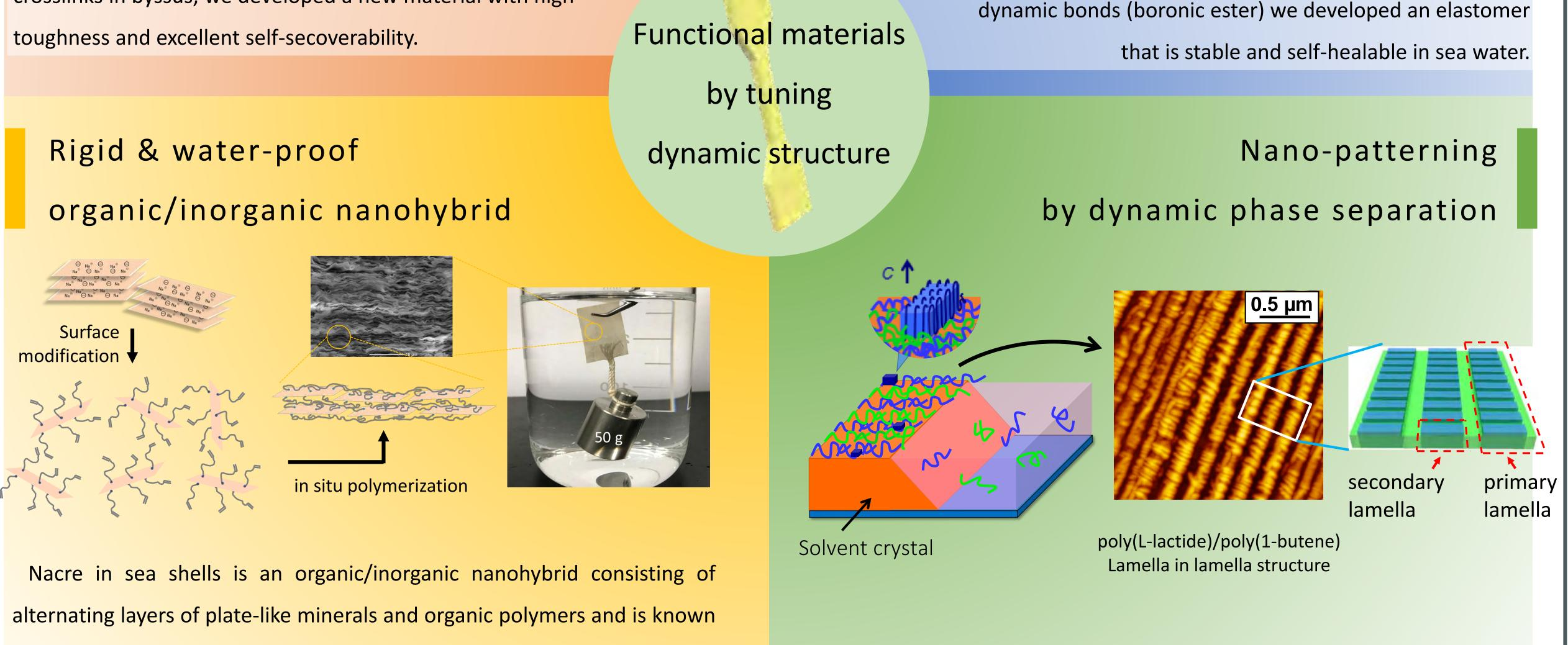
for its high rigidity and low permeability. However, artificial nacre-mimetic materials are often water-sensitive because of high hydrophilicity of the inorganic component. We developed a rigid, water-proof nanohybrid by
