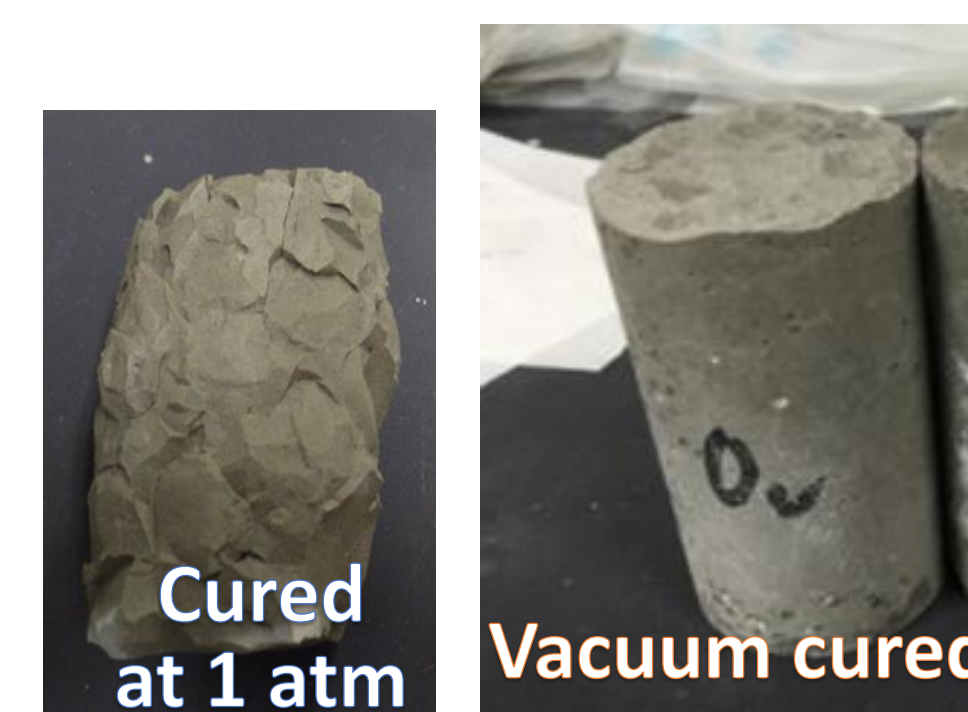
High frost damage resistance after vacuuming
