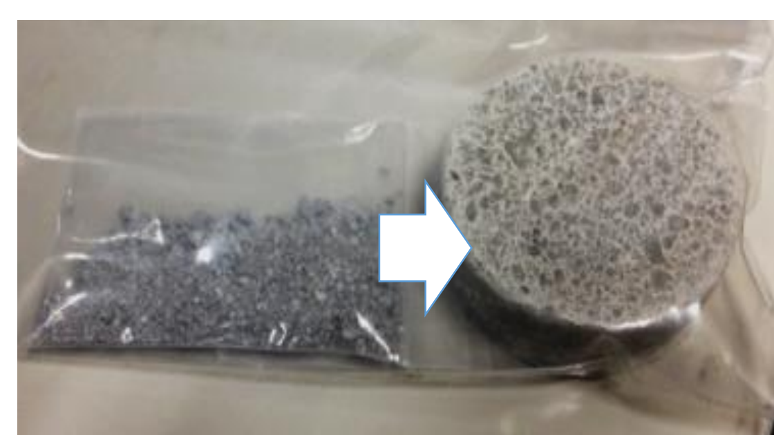
Recycling of crushed concrete
