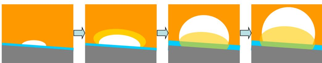
Formation of small cavity due to erosion at some point
