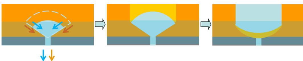
Soil below the ground water level flows with water through the hole. A cavity can expand.
