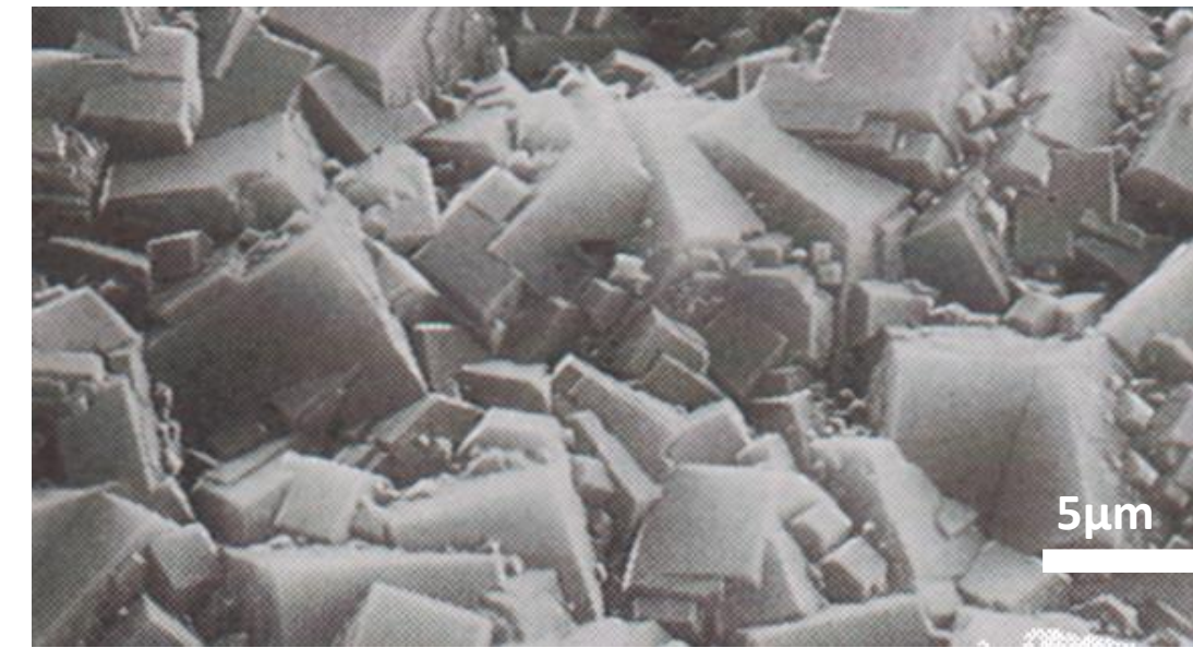
Polycrystalline diamond film. A square (100) can be observed. Since the crystal habits clearly appear, the surface roughness of film is huge.
