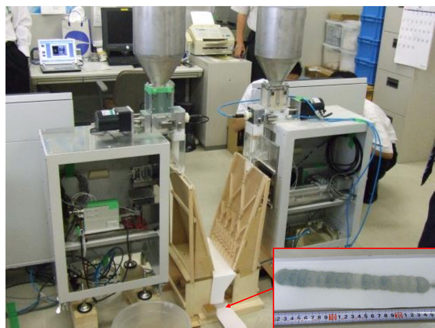
3D mixing system of powder using dividing channel, and mixture of Al 2 O 3 and SiC.
