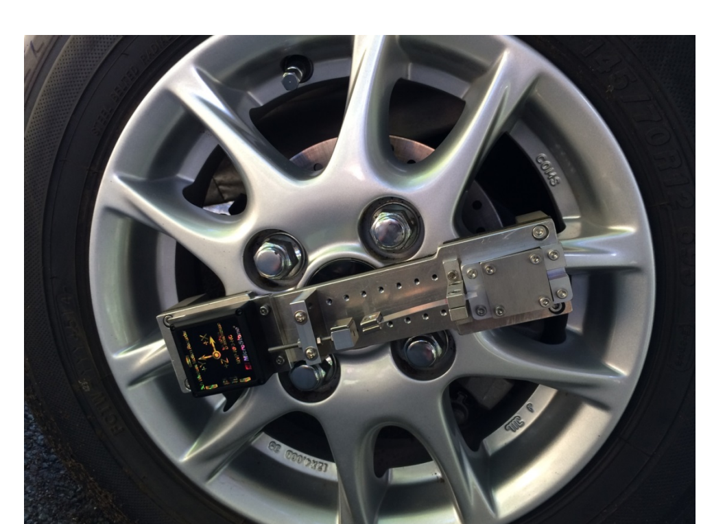
Energy Harvester in the Rotating Tire
