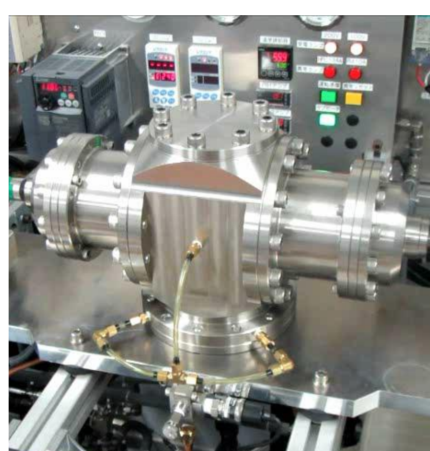
Two phase expander &amp; demonstration unit for trilateral cycle
