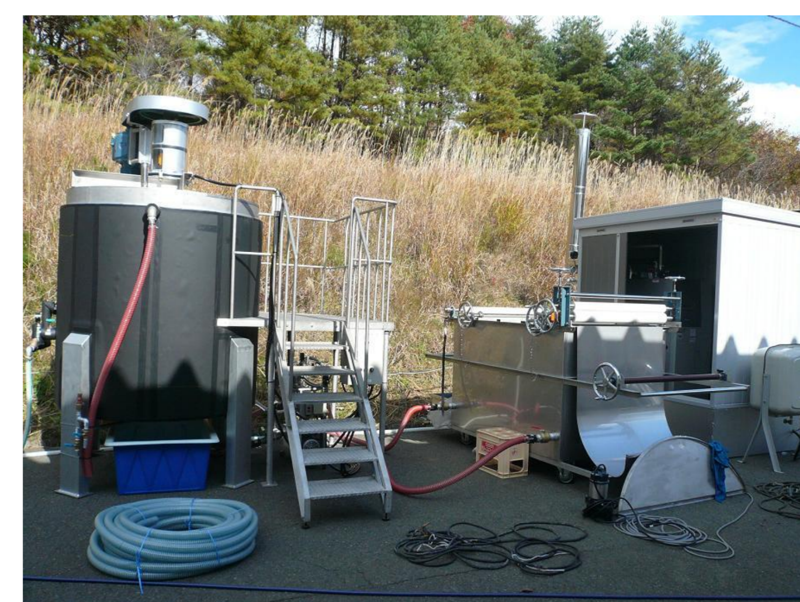
Removal of radioactive cesium from soil by Prussian blue
