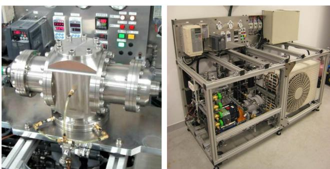
Fig. 5 Expander & demonstration unit for Trilateral steam cycle
