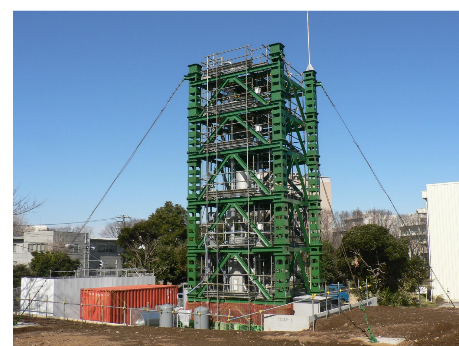
Large scale circulating fluidized bed cold model in Chiba Experimental Station (h: 16 m, d: 0.10 m)
