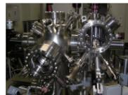
温度可変超高真空STM/AFM
