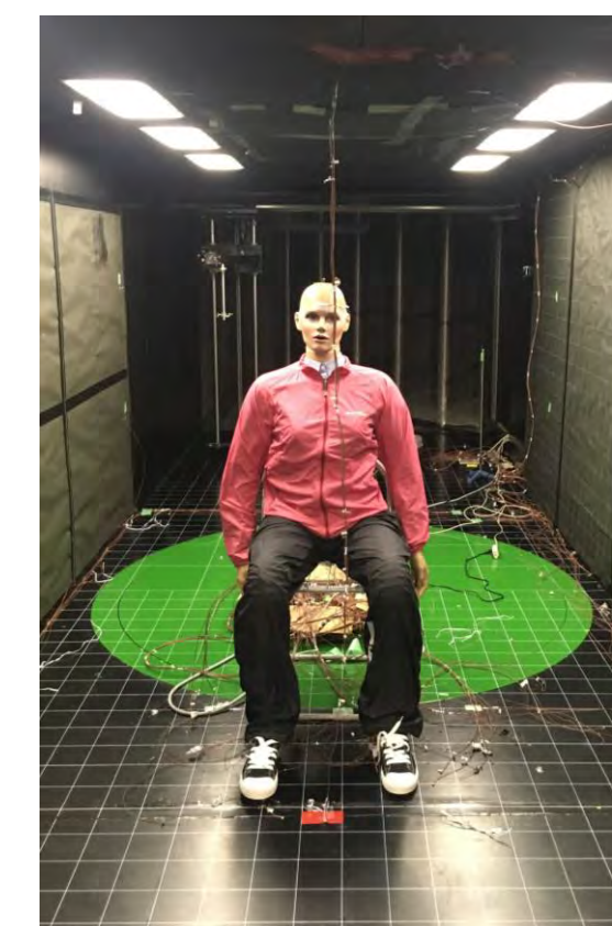
■ Evaluation of thermal environment around human body using a thermal manikin
