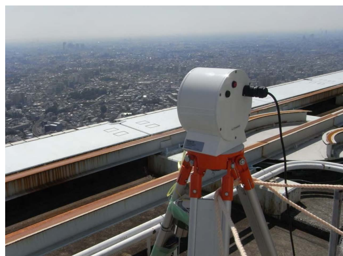
■ Estimation of heat fluxes using Scintillometer
