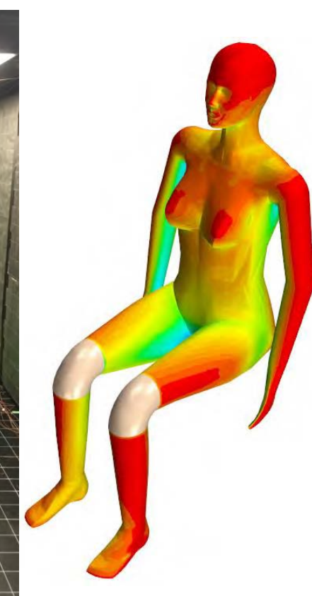
■ Evaluation of thermal environment around human body using a thermal manikin
