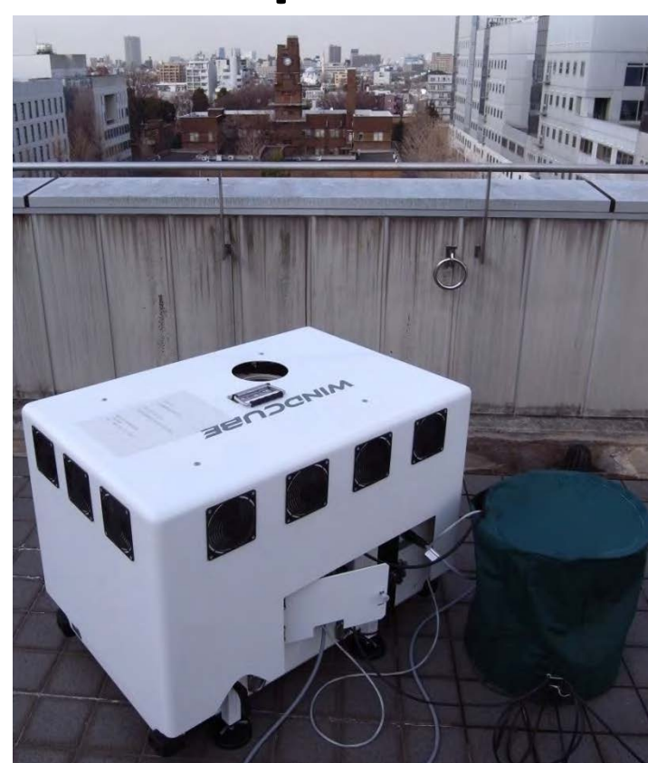
■ Wind velocity observation with a Doppler lidar
