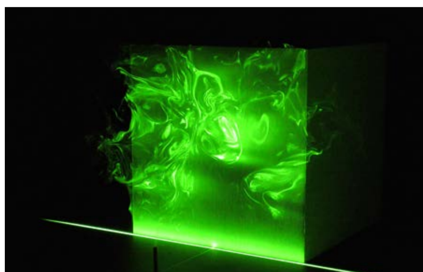
Visualization of pollutant dispersion in wind tunnel
