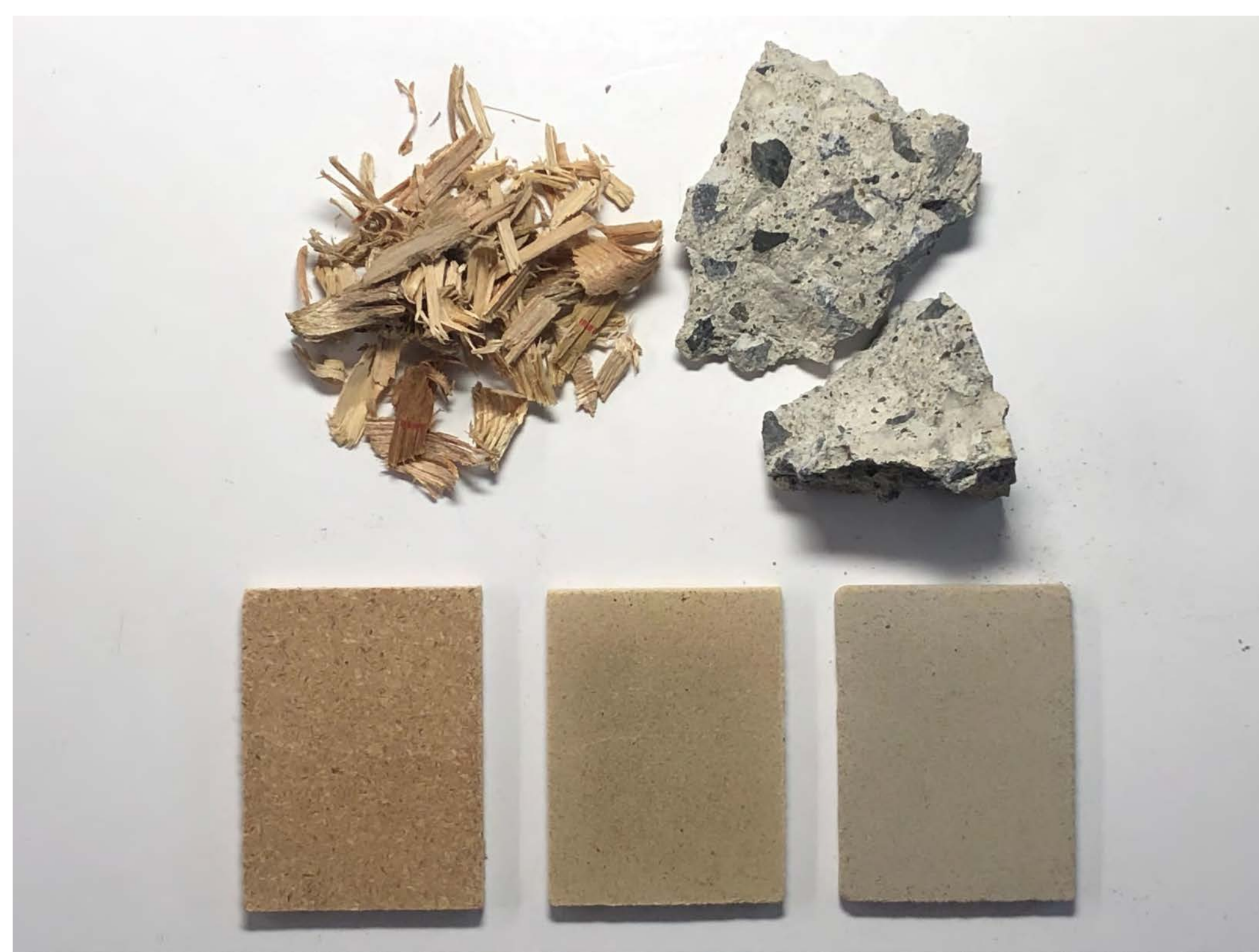
Botanical concrete produced from concrete and wood wastes
