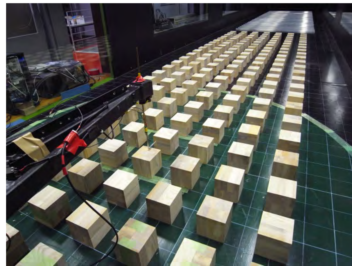
Wind tunnel experiment of city airflow
