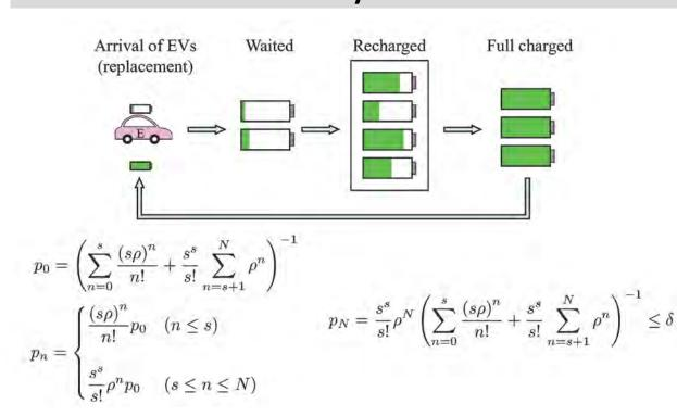
Some company has proposed an EV operations system called 'battery switch system'. In this study, we are focusing on the infra-structure required to support the optimal operation of battery switching system.
