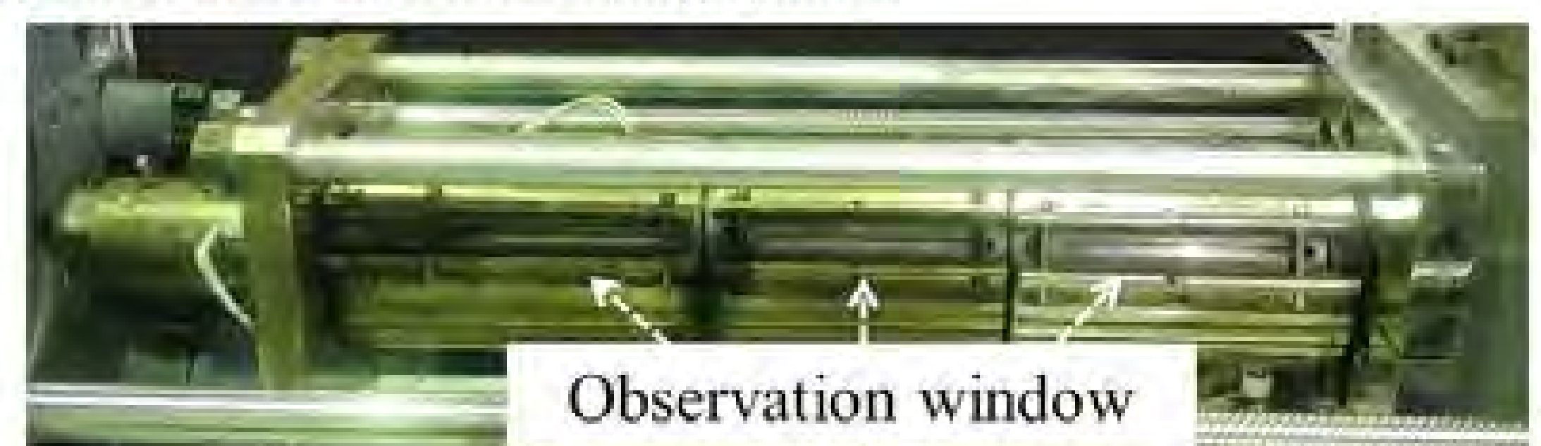
(2) Extended lamination image inside screw channels
