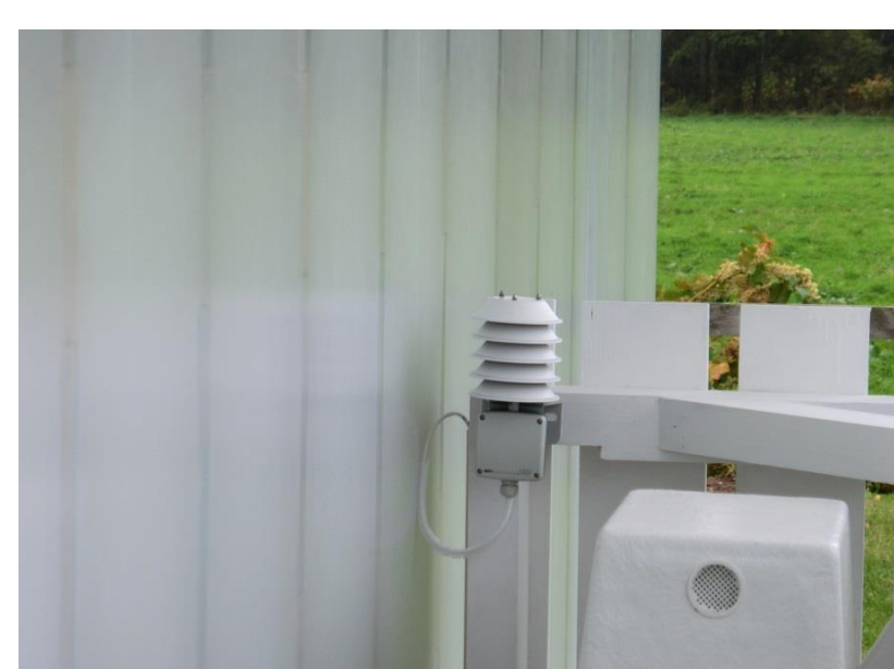
Outside air Thermal and Humidity sensors 外気温湿度計
