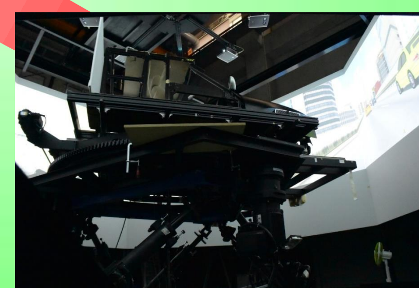
Driving Simulator with 6 d.o.f motion, Turntable & 360° Full Screen
