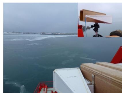
microwave backscattering experiment on icebreaker
