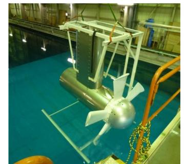
Rotor test in water tank
