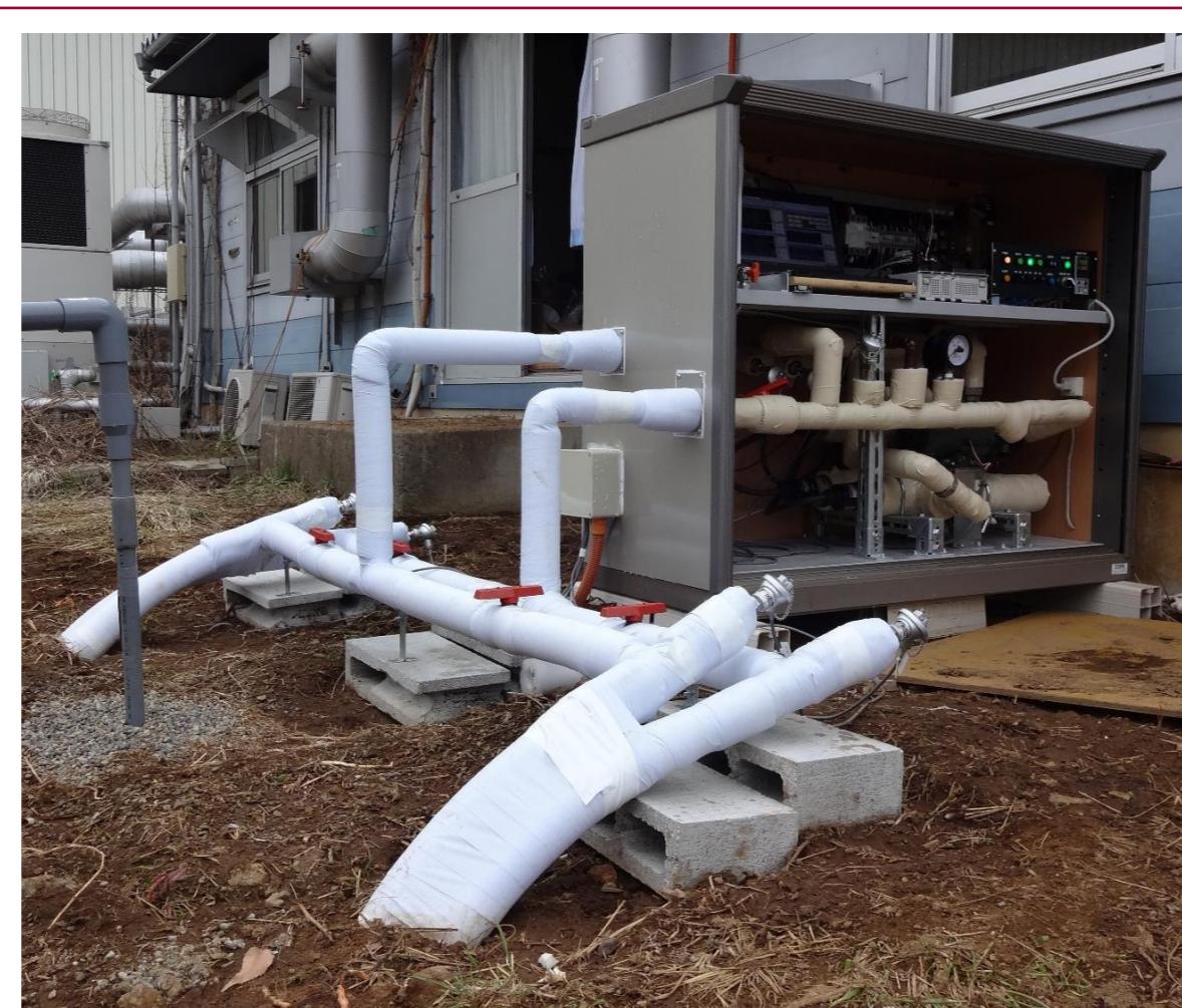
■ Thermal response test experimental system
