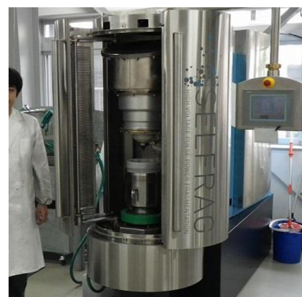
Apparatus of electrical disintegration method using electric pulse
