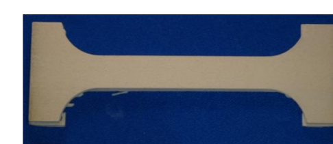
AM product made of high heat-resistant resin
