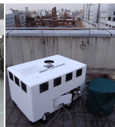
■ Wind velocity observation with a Doppler radar
