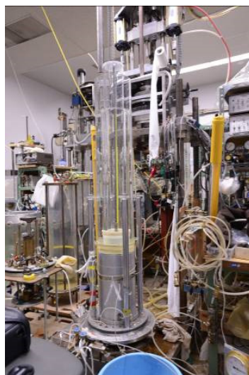
Fig.2 Preparation of segregated specimen by pluviation through water
