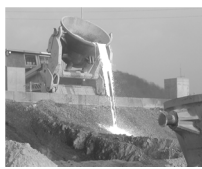
Gradual cooling of steelmaking slag
